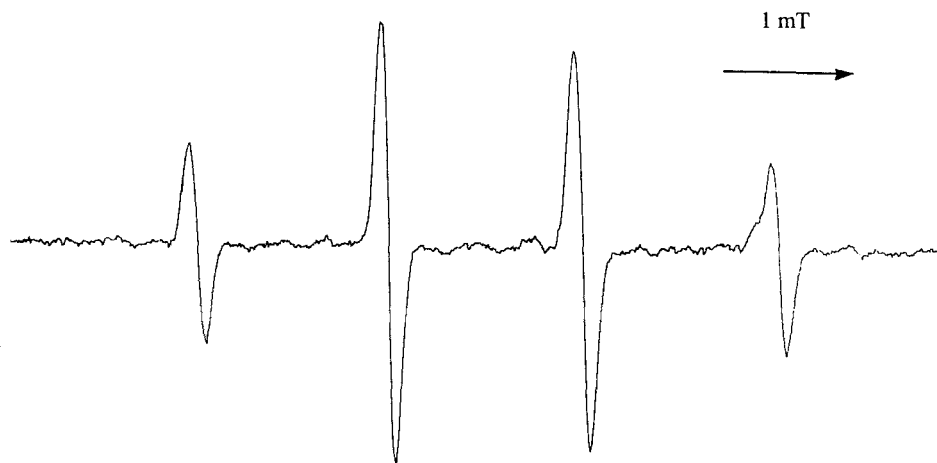
FIGURE 1 E.P.R. spectrum of the hydroxyl-radical adduct of DMPO, generated by reaction of MMPP (0.06 mM) with Staph. A. ( 2 \times 10^9 c.f.u./ml) in the presence of DMPO (66 mM).
